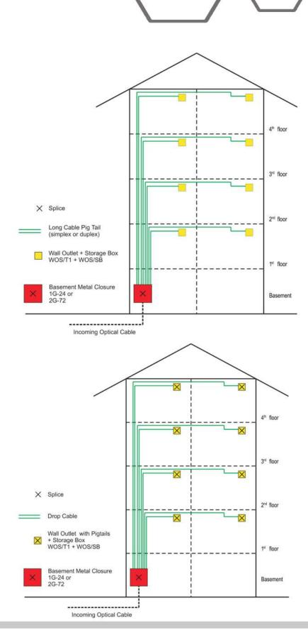
Variant 2: Basement Metal Closure Wall Outlets Fiber Pigtails Drop Cable
